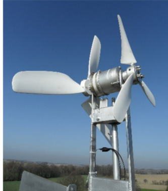
Figure 5.: Unconventional WTs: Dual-Rotor Wind Turbine
