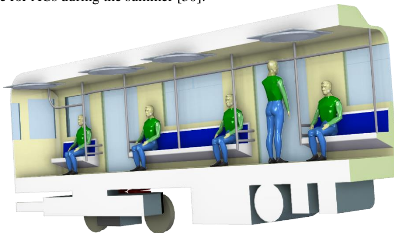
Figure 10. M3 metro train with ACs
