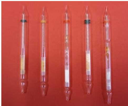
Figure 2: Examples of detection tubes (VFK-66) Source: Compiled by the author.
