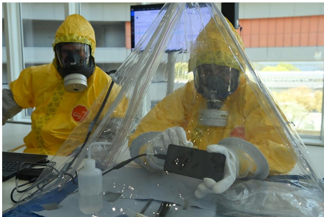
Figure 1: Safe extraction of radioactively contaminated mobile phone data using a UFED tool, while also capturing DNA residue (Photo: D. Calma UN IAEA)
