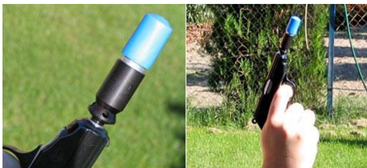
Figure 19: Signal rocket extension with signal rocket [9]
