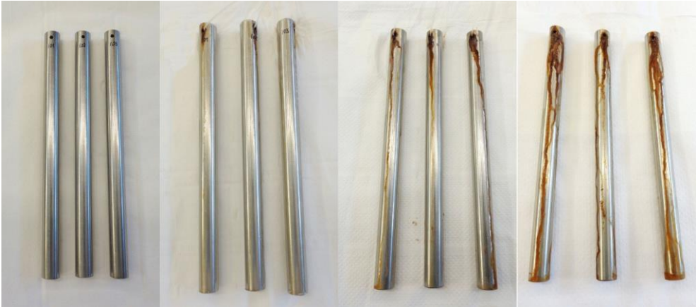
Figure 7. AISI 303 (ground surface finish) samples after 0, 168, 336, and 816 hours. [1]
