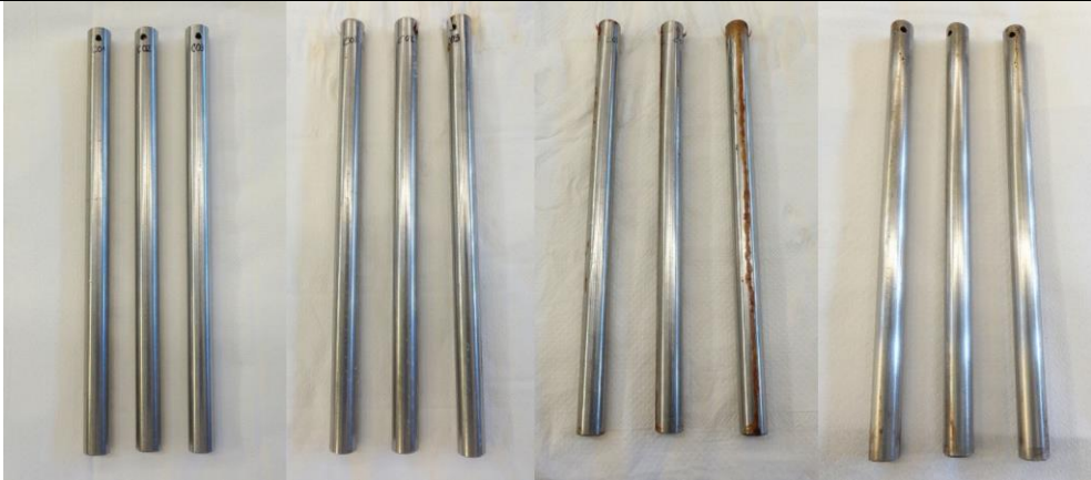
Figure 4. AISI 430 (drawn surface finish) samples after 0, 168, 336, and 816 hours. [1]
