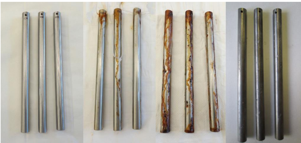
Figure 2. AISI 430F (ground surface finish) samples after 0, 168, 336, and 600 hours. [1]
