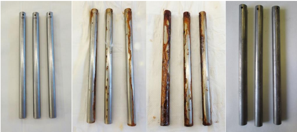
Figure 1. AISI 430F (drawn surface finish) samples after 0, 168, 336, and 600 hours. [1]
