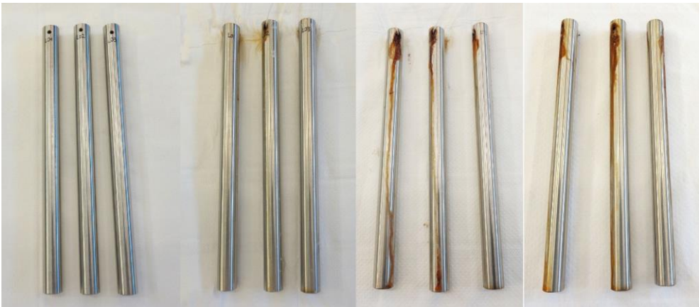
Figure 8. AISI 303 (ground surface finish) samples after 0, 168, 336, and 816 hours. [1]
