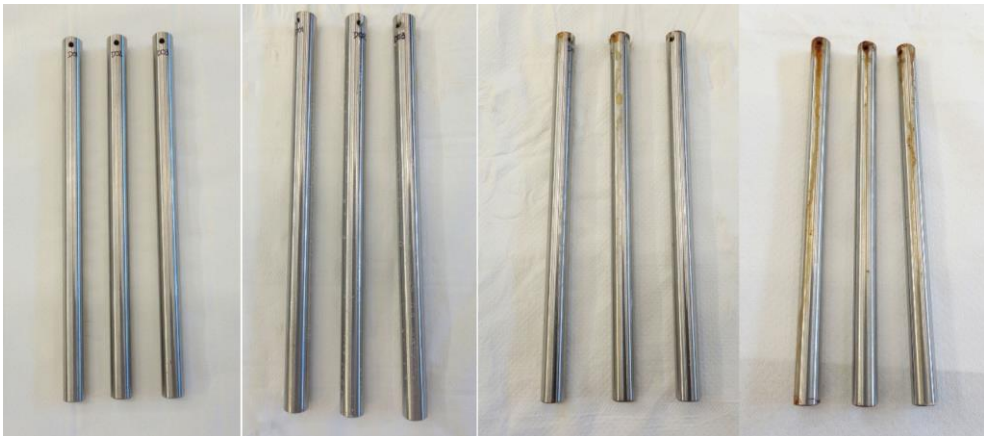
Figure 5. AISI 430 (ground surface finish) samples after 0, 168, 336, and 816 hours. [1]
