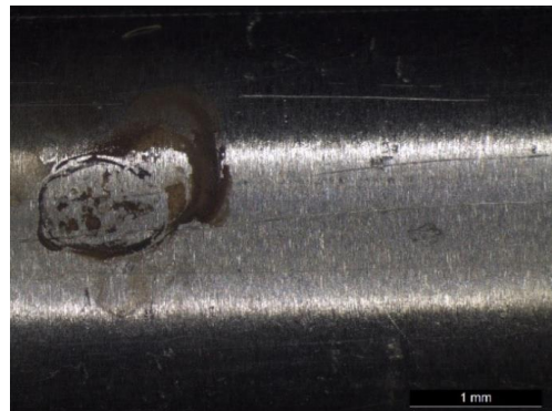
Figure 6. Microscopic image of AISI 430 drawn and ground surface samples [1]
