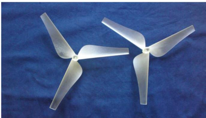
Figure 10. 3D printed turbines
